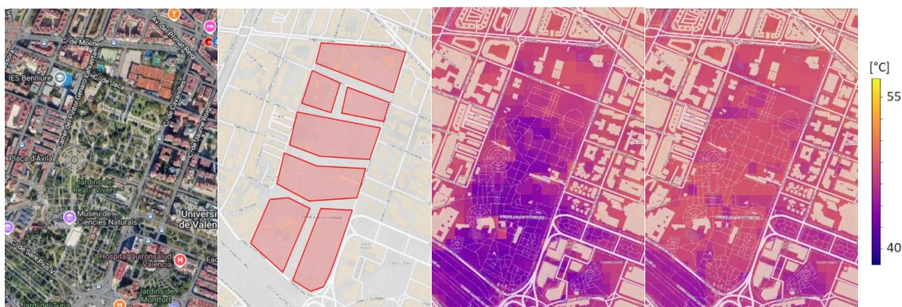
Figure 8. Example for performance of the EO-based Heat Island Simulation and Mitigation Strategies Service Engine. Sealing the municipal park Jardins del Real in Valencia, Spain, leads to an increase of about 4.4 °C over the modified areas. The simulation was done for the extreme summer day of 2023 (model  $R^2$  of 0.57, RMSE of 0.66K).
