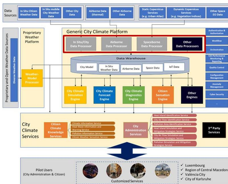
Figure 1. The components of WP5 “Data Processors for City Weather Model” (red box) within the CityCLIM architecture.
