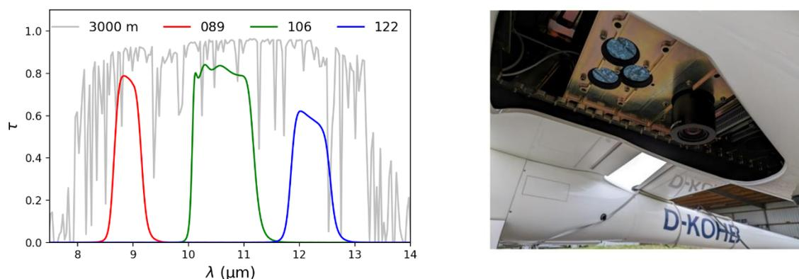
Figure 4: Spectral bands of the sensor “RAVEN” and simulated atmospheric transmittance (left). RAVEN and high-resolution RGB camera as integrated in the airborne system.
