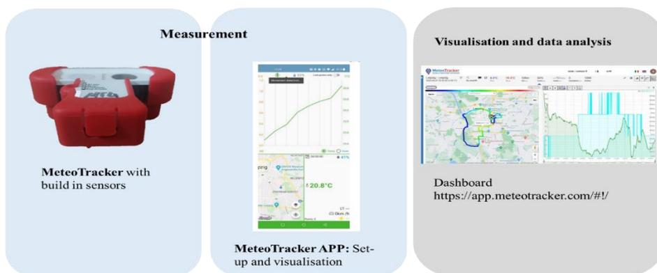
Figure 7: Components of the MeteoTracker sensor solution: sensor, app and dashboard
