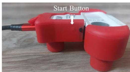
A short press on the start button switches the unit on and off. Pressing the button for more than 10 seconds will reset the settings. The RESET status lights red.
