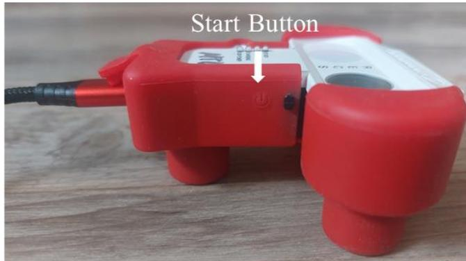
1. A short press on the start button switches the unit on. The yellow BT ADV LED is flashing meaning that the device is switched on and is searching for a Bluetooth connection with a smartphone
